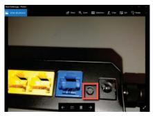
The Power Port is underlined in Red, it is at the edge of one of the side, near the one of the 4G antennas
