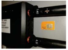
The SIM card snaps in the slot thanks to a spring system. The image below shows when the card is inserted correctly.
