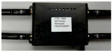
Please refer to the picture above to mount the antennas with utmost care. The router has 4 antennas, 24g and 2 wifi.
