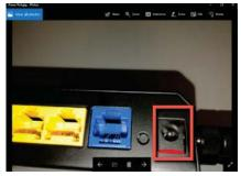
The Blue Ethernet port is to be used ONLY when the host location is providing us with a hardline connection. The Host location's internet supply line will come to us via this blue port.
