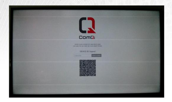
Use the remote and the Content Home button. Select the URL Launcher and the ComQi EEP commissioning page should be visible on the screen.
