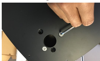
Attach large base leaving small plate in-between the base plate and stand using an Allen wrench
