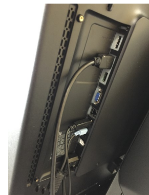
Newer ELO screen models will have their cable and power source connections vertically accessible on the back side of the screen.
