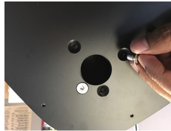
Attach large base leaving small plate in-between the base plate and stand using an Allen wrench
