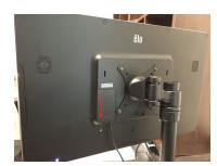
Slide off the rectangular panel on the back of the tablet
