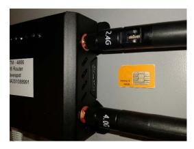
The SIM card snaps in the slot thanks to a spring system. The image below shows when the card is inserted correctly.
