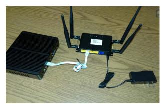
Please refer to the picture below to mount the antennas with utmost care. The router ha 4 antennas, 2 4g and 2 wi-fi. The 4G antennas come with a contact pin while the wi-fi ones don't. The wi-fi antennas' contact pins are located inside the ports. So, it is important to always look inside a port and determine which antennas goes in before inserting and tightening. Notice that alike antennas are set up across each other on the same side of the router.
